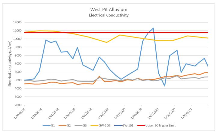
Figure 63 - West Pit Alluvium Electrical Conductivity Trend - Q1 2021
