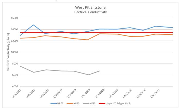
Figure 66 - West Pit Siltstone Electrical Conductivity Trend - Q1 2021
