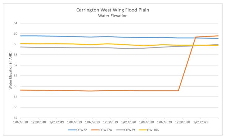
Figure 47 - Carrington West Wing Flood Plain Water Elevation Trend - Q1 2021
