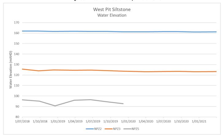
Figure 68 - West Pit Siltstone Water Elevation Trend - Q1 2021
