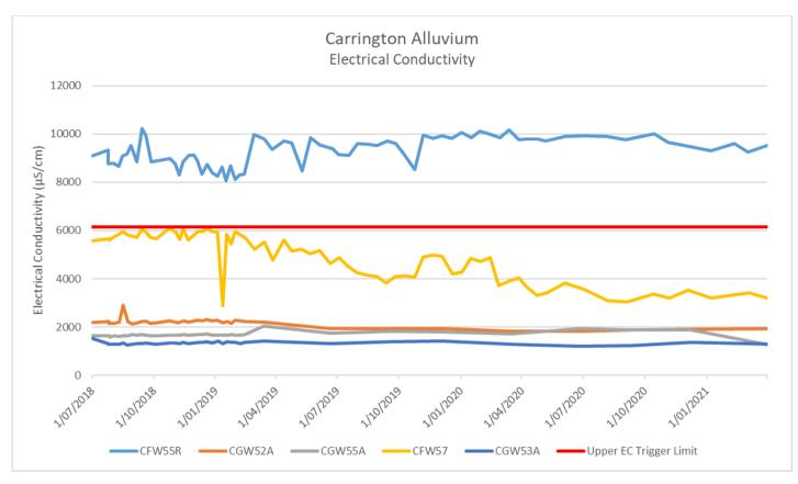
Figure 27 - Carrington Alluvium Electrical Conductivity Trend - Q1 2021
