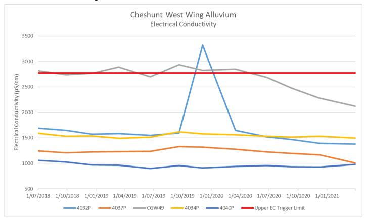
Figure 42 - Cheshunt West Wing Alluvium Electrical Conductivity Trend - Q1 2021
